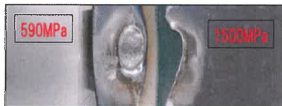
Tensile Test Results of Welded 1,500 MPa Steel
