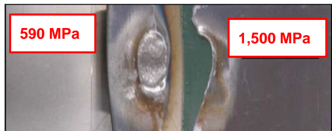
Tensile Test Results of MAG-Welded 1,500 MPa Steel
