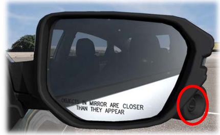
LaneWatch Camera Location
