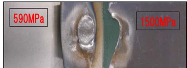
Tensile Test Results of Welded 1,500 MPa Steel
